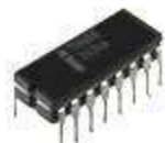
Puce au format DIP ( Dual In-line Package )
